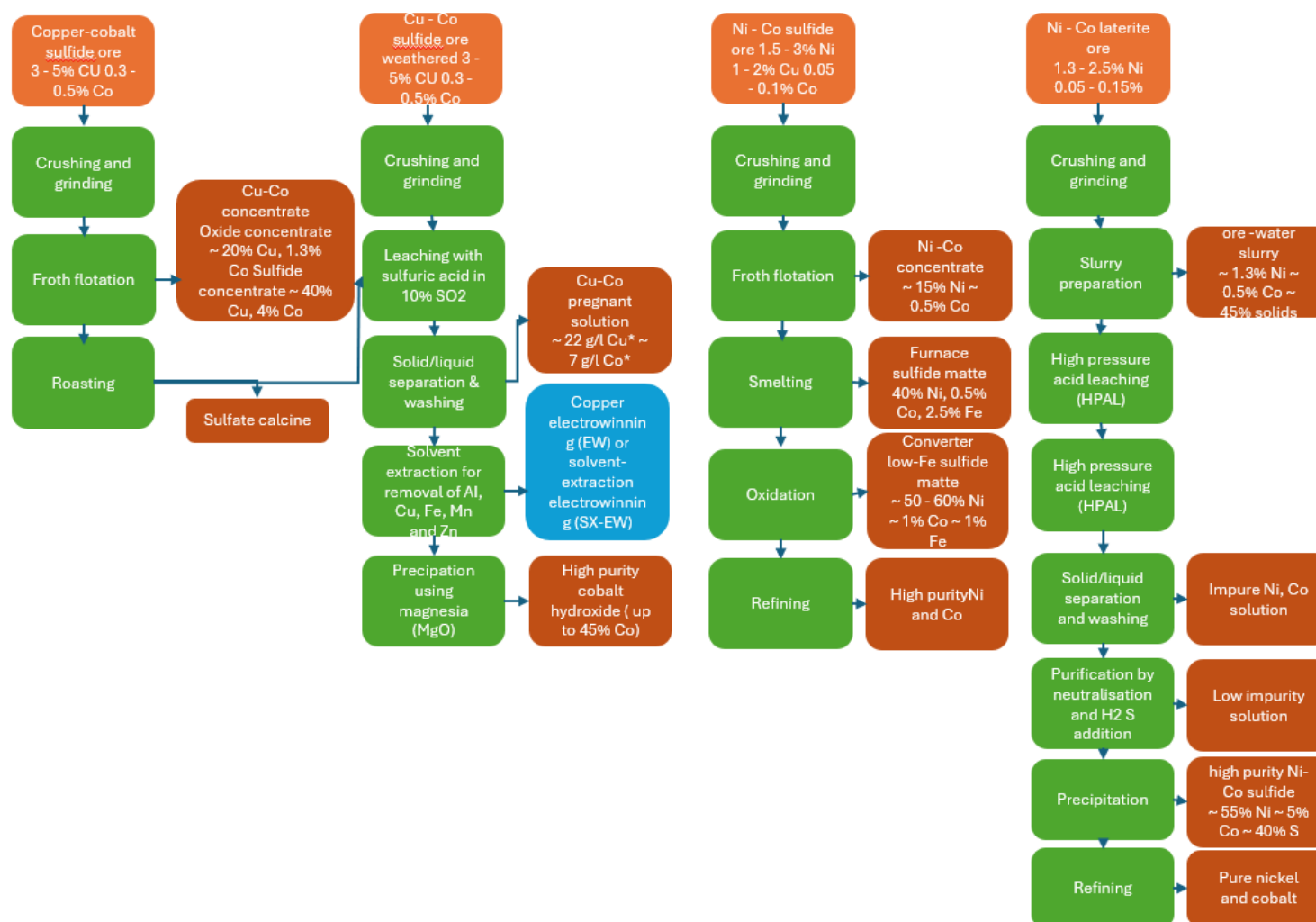
Figure 6: Cobalt processing steps for three types of ore: copper-cobalt sulfide ore, nickel-cobalt sulfide ore and nickel-cobalt laterite ore, adapted from (Petavratzi et al. 2019)
